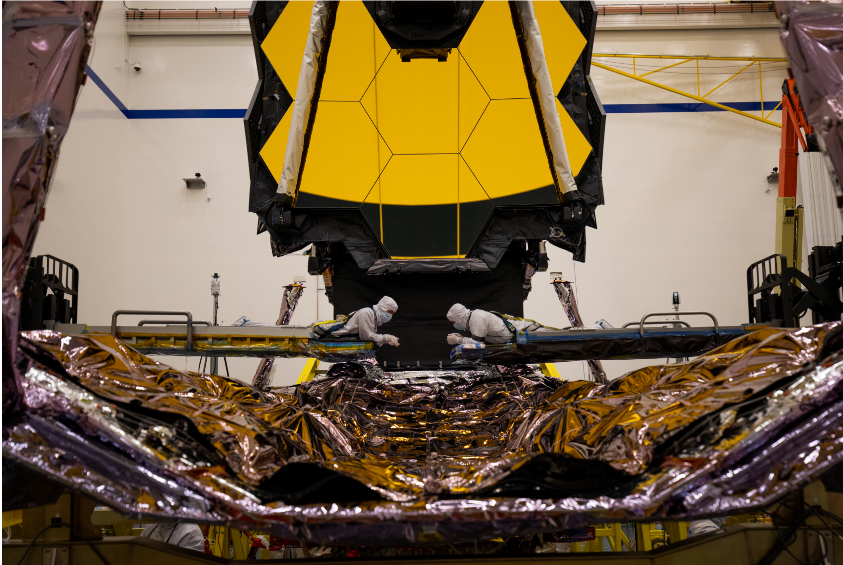
JWST Deployable Tower Assembly extension (June 2020). Credit: Northrop Grumman https://www.nasa.gov/feature/goddard/2020/tower-extension-test-a-success-for-nasa-s-james-webb-space-telescope
