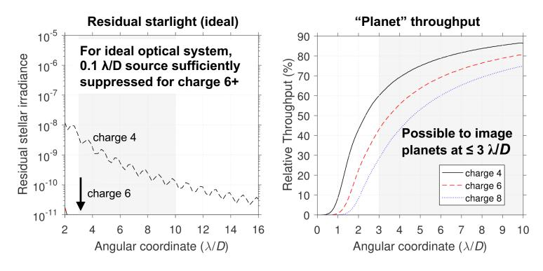
Stellar irradiance is azimuthally averaged and normalized to the peak of the telescope PSF.
