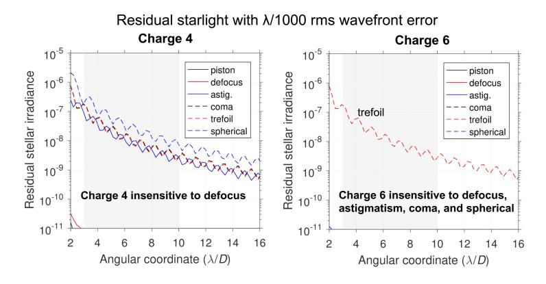
Stellar irradiance is azimuthally averaged and normalized to the peak of the telescope PSF.
