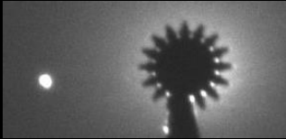
Suppressing scattered light off petal edges from off-axis Sunlight (S-2)
