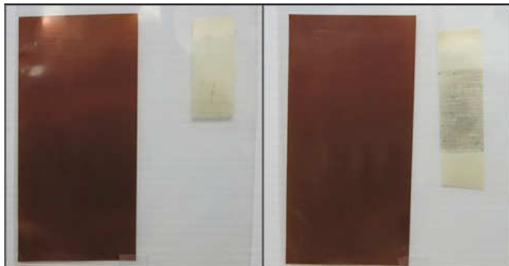
Figure 3-10: Adhesion test results after cyclic abrasion testing for the Acktar (left) and Enbio (right) coupons. Both the Kapton surface used for abrasion (copper colored material) and the tape are shown.
