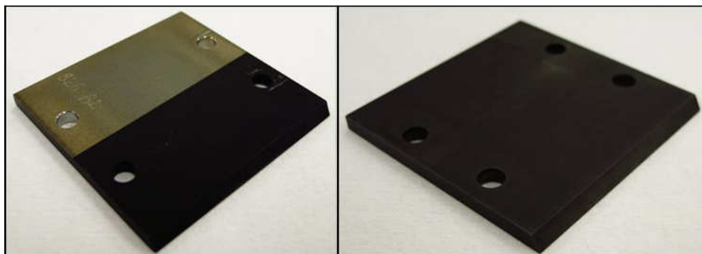
Figure 3-11: Visual inspections of the Acktar (left) and Enbio (right) coupons after thermal cycling and humidity exposure. No effects were observed.
