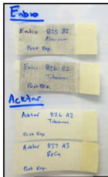
Figure 3-12: Adhesion test results after thermal cycling/humidity exposure for the Acktar (bottom) and Enbio (top) coupons.
