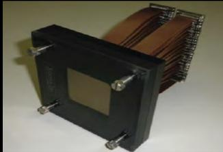
CG-16: Cryogenic Deformable Mirror
