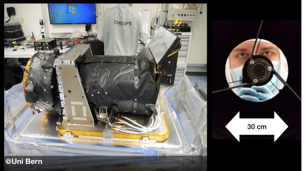
A 30-cm space telescope capable of ultra high-precision photometry
