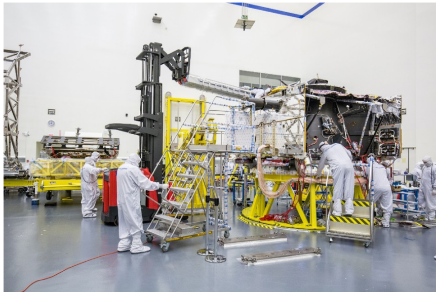
Second sunshield mid-boom installation
