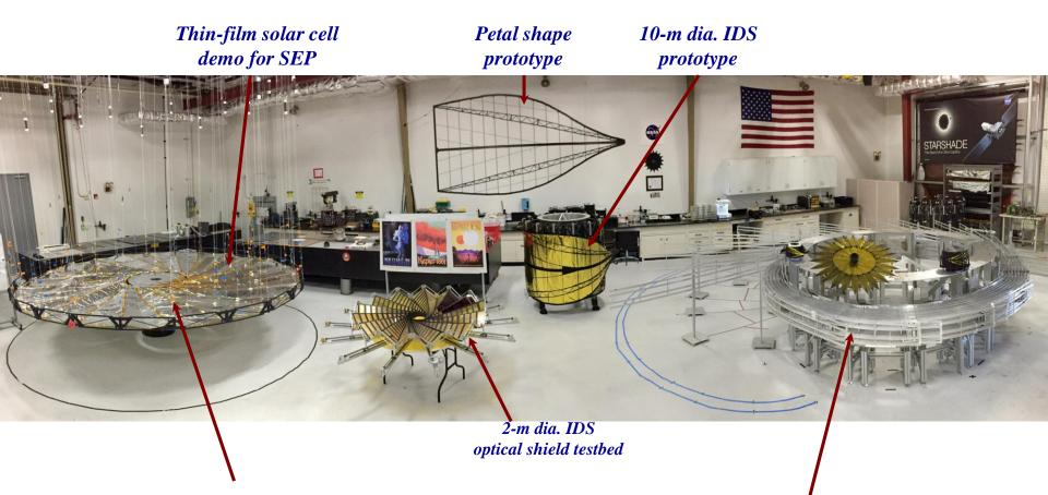
Established 5-m dia. IDS optical shield testbed to: Develop truss closeouts, incorporate carbon rods at all OS hinge lines, demo thin-film solar cells.
