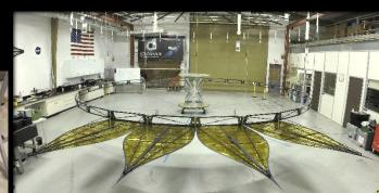
Positioning the petals to high precision, blocking on-axis starlight, maintaining overall shape on a highly stable structure (S-5)
