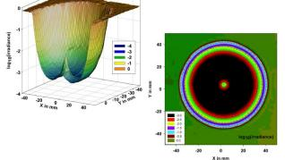
f) Photometer mapping of shadow from 16 petal silicon starshade in white light shows suppression of several orders of magnitude of irradiance within a few millimeters, with an ultimate suppression level of  $< 1 \times 10^{-7}$ .
