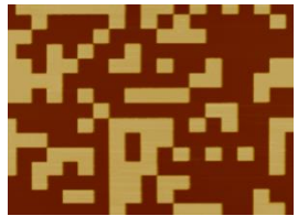
Figure 1. Microscope image (above) and AFM profile (below) of a micro dot patterned mask for JWST NIRCam coronagraph
