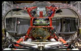
LBTI instrument (green structure) mounted between the two LBT primary mirrors
