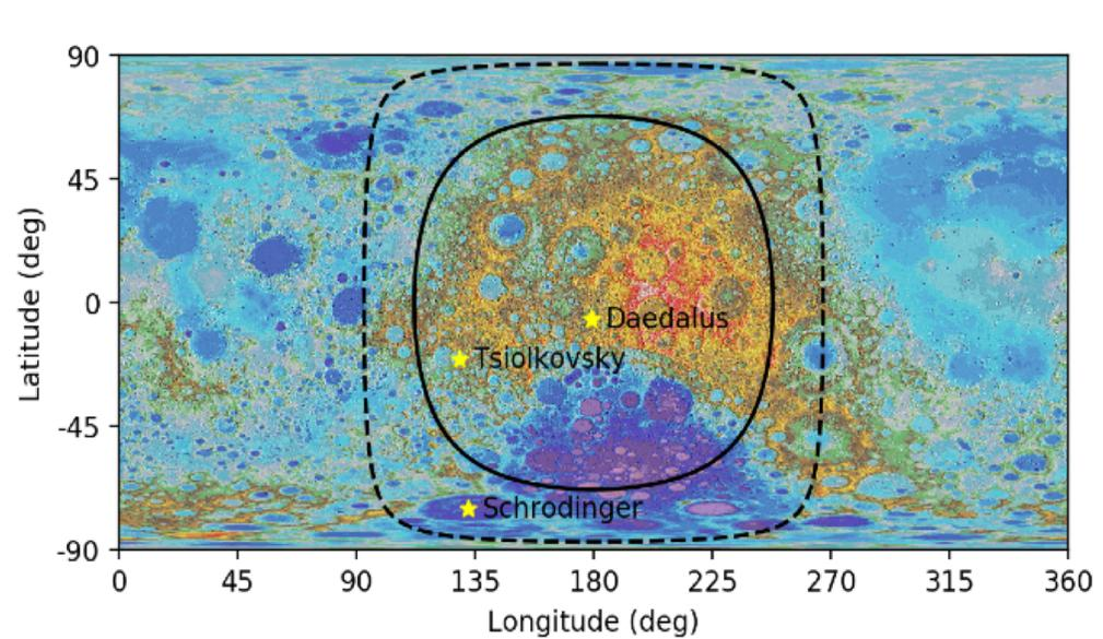
The “radio quiet” region at 100 kHz (solid) and 10 MHz (dashed) defined by  $\geq 80$  dB attenuation plotted over a map of the lunar surface.
