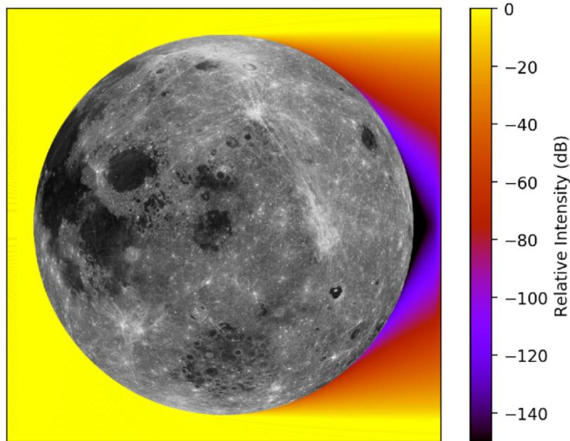
Two-dimensional numerical electrodynamics simulations show that the relative intensity of terrestrial radio waves incident on the Moon is highly attenuated behind the farside.
