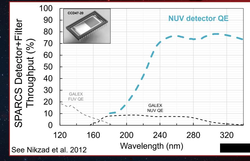
SPARCS' Technology Mission: Fly high-QE, delta-doped detectors (SPARCam) Fully-processed thinned CCDs are modified for UV enhancement by growing 2.5 nm of boron-doped silicon on the back surface.
