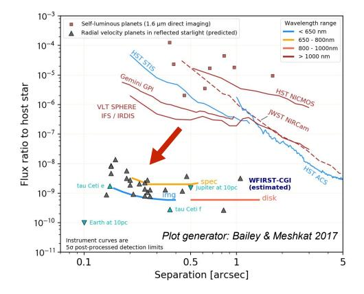
*Early estimates of the CGI flux ratio curves* for three observing configurations (direct imaging at short and long wavelengths, and integral field spectroscopy) are based on *currently demonstrated static and dynamic testbed performance* and observatory optical disturbance models provided by the WFIRST project.
