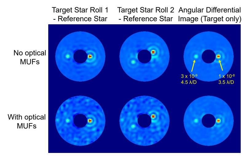
Field incident on detector shown. Detector effects not included
