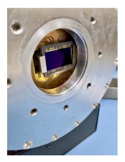
e2v 1K X 1K Electron Multiplying CCDs For all cameras, running at different modes
