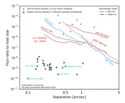
Direct imaging and spectroscopy of **young self-luminous exoplanets** have been achieved from ground and space observatories. Direct imaging of **mature cool exoplanets in reflected starlight** is currently beyond the reach of conventional techniques, as illustrated by the estimated brightness of a sample of known radial velocity exoplanets.
