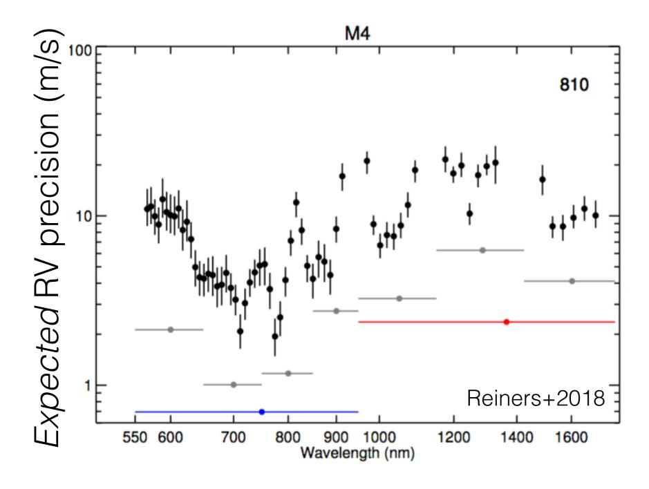
Carmenes spans optical and NIR - direct comparisons possible Trade-off: S/N (†NIR) vs. spectral content (†optical)
