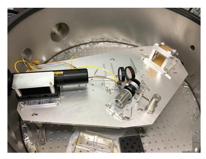
Single-mode fiber input R~50,000; 840-920 nm High throughput milli-Kelvin temperature stability Mostly "off the shelf" parts
