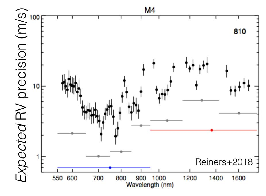
For almost all M dwarfs, 700 nm to 900 nm appears optimal Caveats: Intrinsic stellar RV noise could be much better in NIR Dealing with telluric lines in RV analyses
