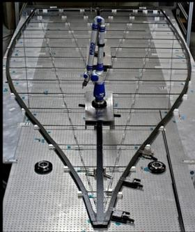
(4) Sub-scale test demonstrating lateral formation sensing accuracy
