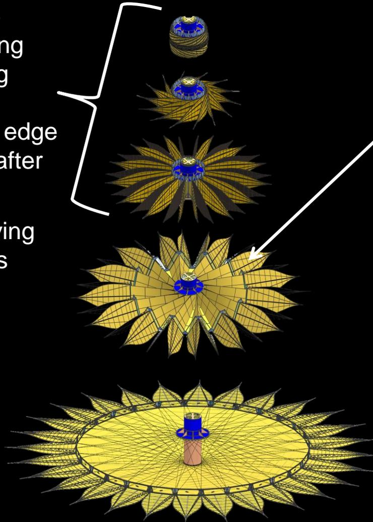
(3) half- to full-scale deployment and petal positioning mechanisms
