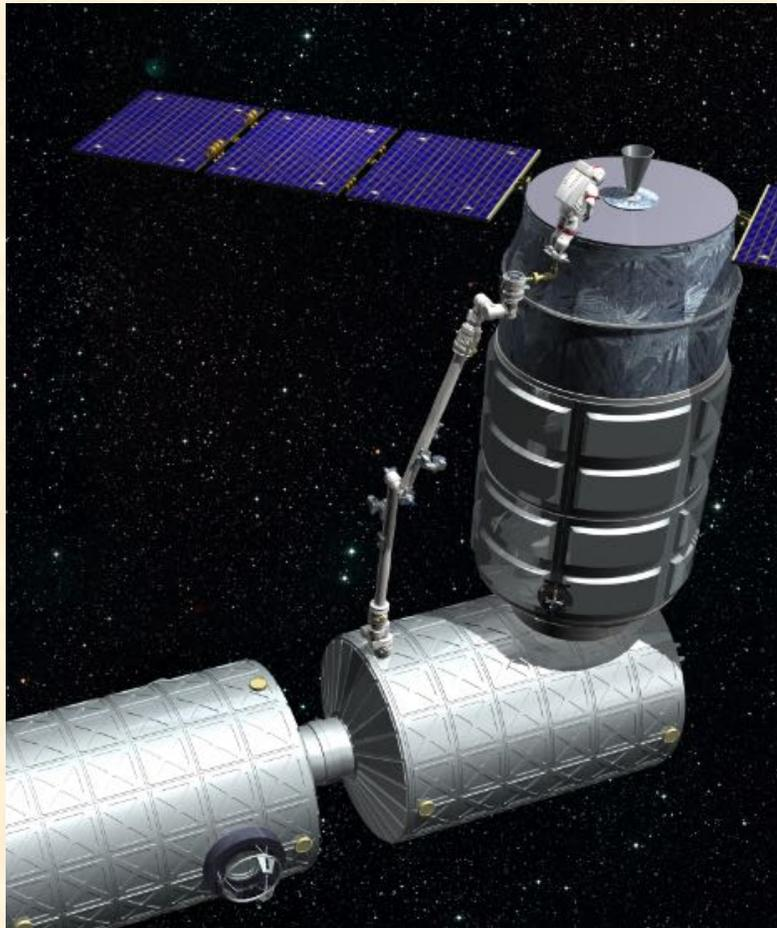
A habitation and operations site in cislunar space will require a highly capable robotic arm.
