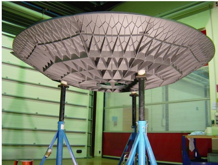
Figure 20: The Herschel telescope primary mirror with ribbed backstructure 23
