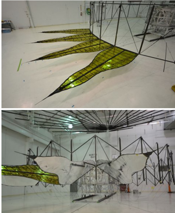
Figure 9.5-1. Deployed position tolerance demonstration. Petal root positions are measured after each of 20 deployments.
