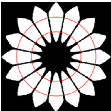
Figure 9.2-1. Starshade test article supported by a diffraction controlling outer ring. Red circles indicate the inner and outer working angles.
