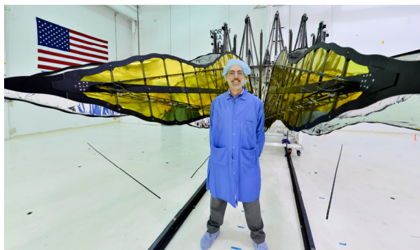
Figure 1.2-3. Starshade stowage and deployment test with four petals and a 1 st generation starshade truss. JPL/Princeton/NGC.
