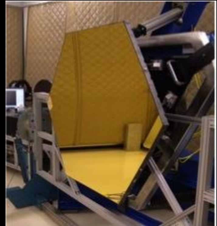
Active Hybrid Mirror (AHM) SiC- based Mirror Segment (AOA/Xinetics/JPL)
