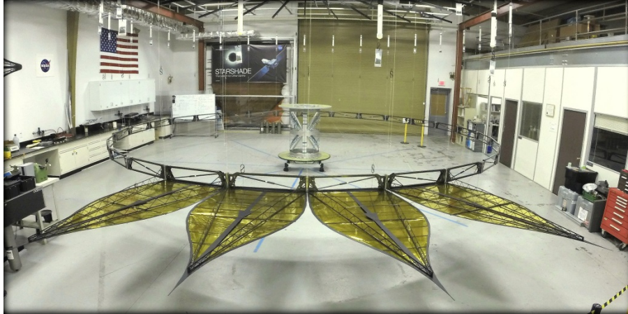
Figure 18: A 10 m inner disk subsystem prototype demonstrates deployment from a stowed configuration and final positioning of the starshade petals. The testbed also allows for studying the petal-inner disk interface. The entire testbed has its weight offloaded by a gravity compensation system. (Image: JPL/Caltech)
