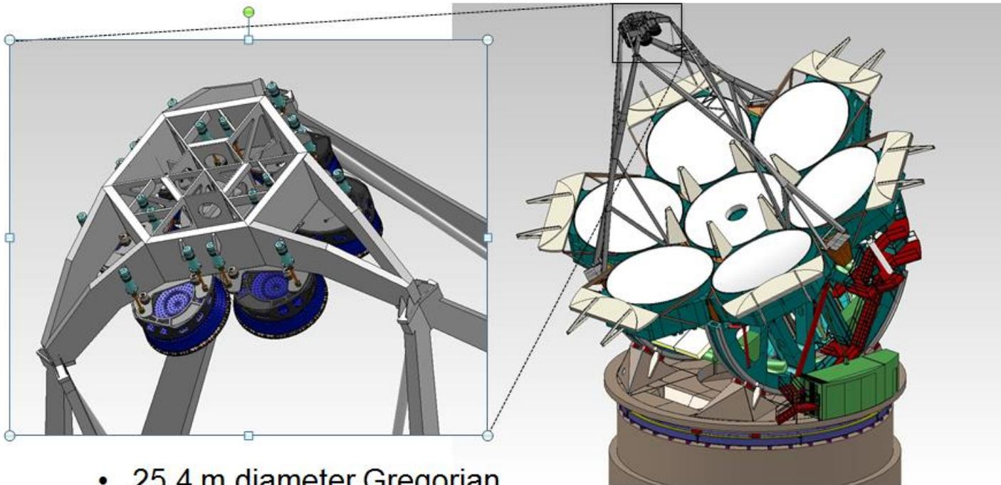
Note: M1 and final M2 system use optical edge sensing
