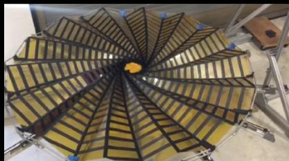
Positioning the petals to high precision, blocking on-axis starlight, maintaining overall shape on a highly stable structure (S-5)
