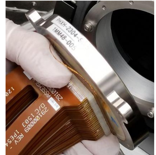
A 48x48 PMN DM, with (non-flight) pins on the back side connecting to flex-print cables
