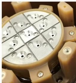
**Figure 14.** CMT extractor electrode.
