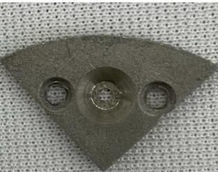
Figure 10. Single emitter assembly porous extractor.
