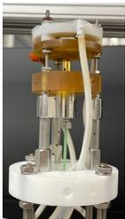
Figure 9. Single electro spray emitter assembly.
