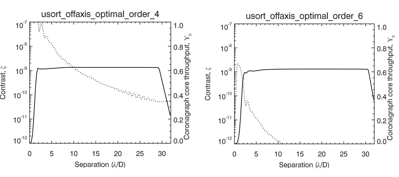
Example Results: USORT off-axis, 6.5m ID, Optimal Coronagraph Limits
