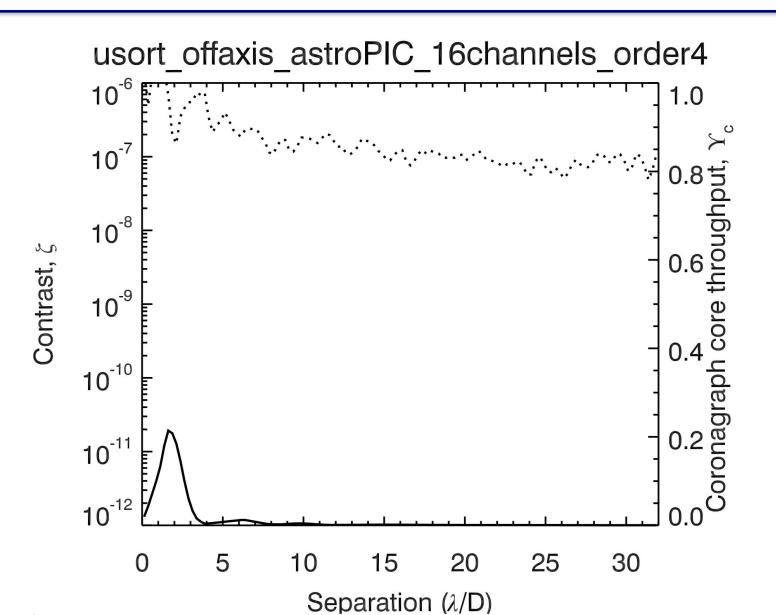
Example Results: USORT Off-axis, 6.5 m ID, 16-channel PIC
