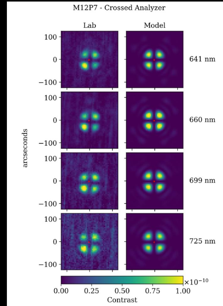
These lobes are entirely due vector diffraction at the miniature starshade edges. Models take into account sub-micron structures on the edges, material properties, polarization.
