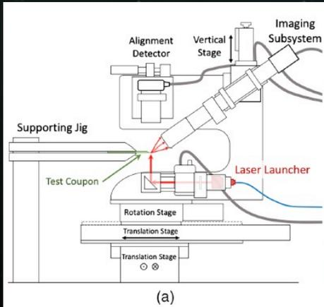
Fig. 6 (a) Schematic of the single-angle scatterometer and (b) picture of the assembled instrument.
