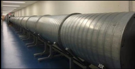
Suppressing scattered light off petal edges from off-axis Sunlight
