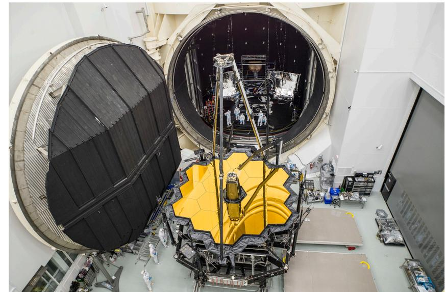
Telescope emerges after cryogenic testing at NASA/JSC
