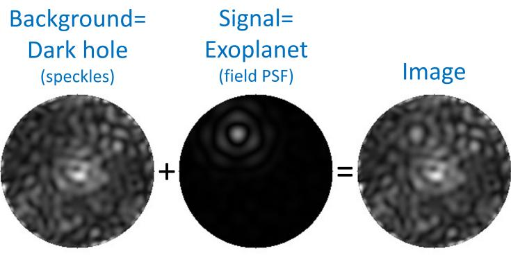
Dependencies: Coronagraph masks Optical errors Polarization aberrations Wavefront correction (DMs) Pointing errors (jitter) Finite-diameter star Dependencies: *Coronagraph masks Optical errors Wavefront correction (DMs)*
