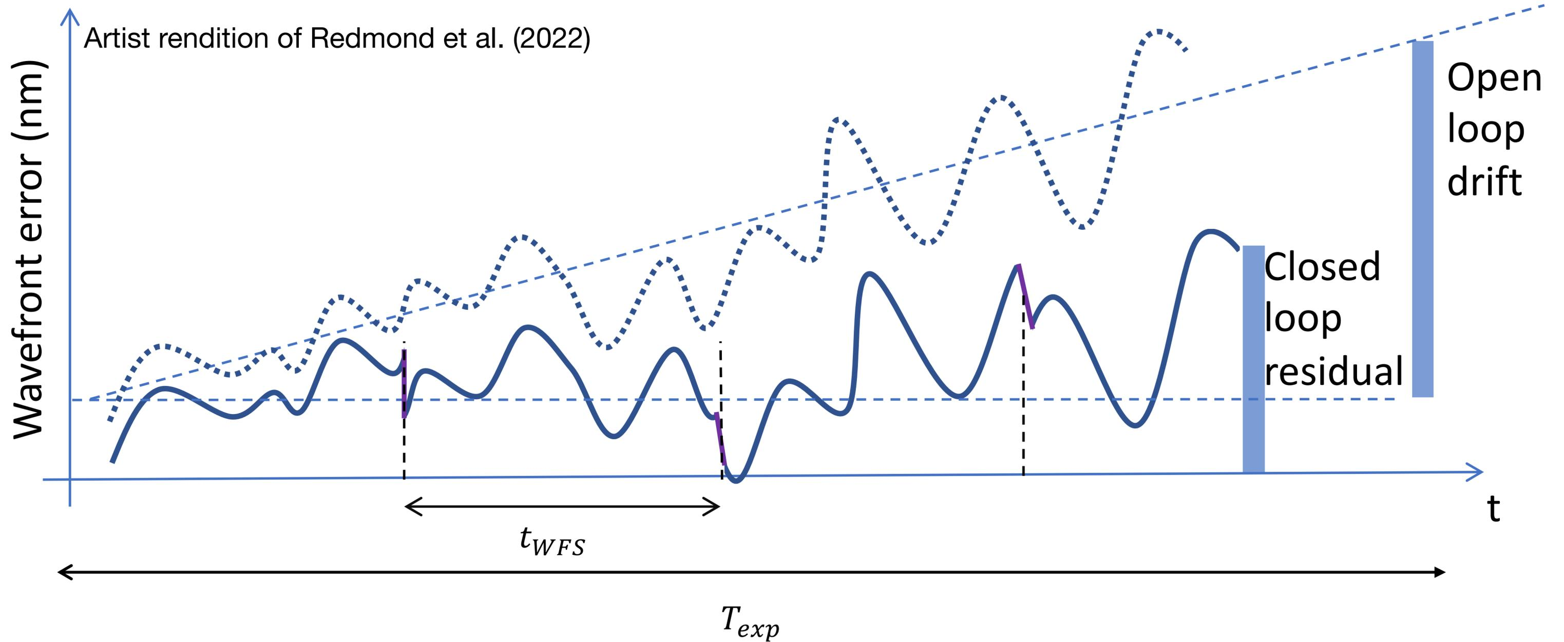
**Shorten the time scales of wavefront drifts from a science exposure time (~10 hours) to a wavefront sensing exposure time (minutes, seconds, milliseconds?).**
