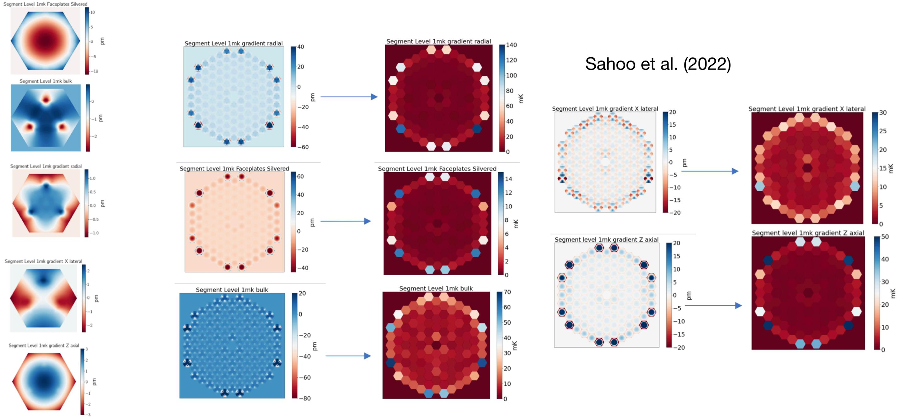
**We find that thermal drifts requirements are of ~5 mK over timescales of 10s of seconds to minutes**
