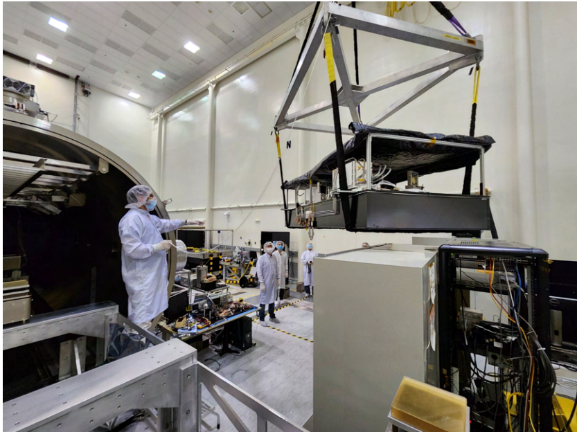
Figure B.3: The DST 2 – a second ultra-stable vacuum coronagraph testbed bench being installed in a vacuum chamber at the HCIT facility. The testbed is being commissioned in late 2022 and will be available to investigations in 2023.
