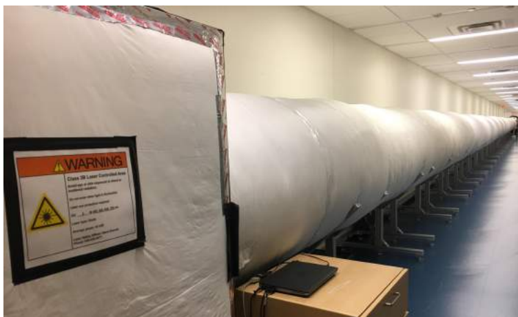
Figure 1: Princeton Starshade Testbed with newly installed 2" thick fiberglass insulation covering the 78 m long tube.
