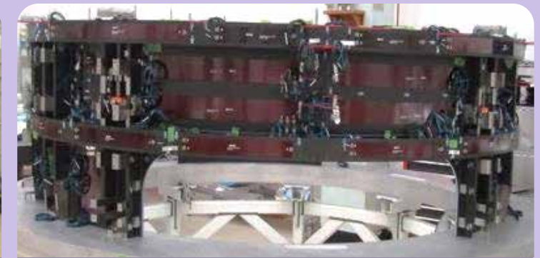
Forward Metering Shell w/thermal control hardware installed
