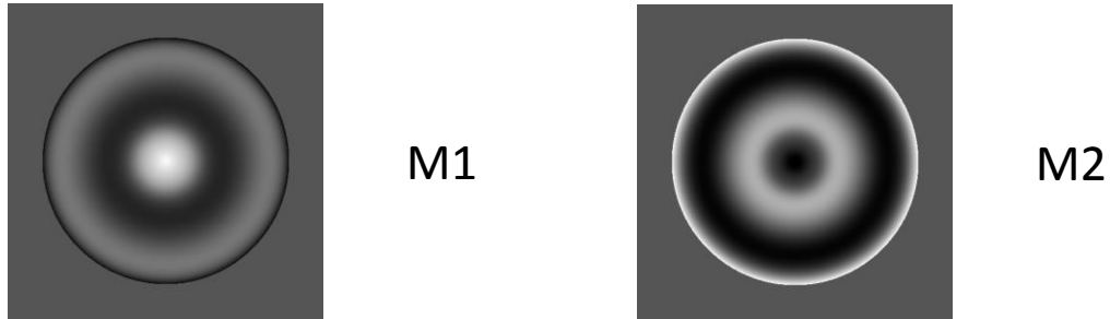
Fig. 2. Aspheric components of Gen 2 PIAA mirror shapes. The P-V deviation from a conic surface is 2.1 \mu\text{m} .
