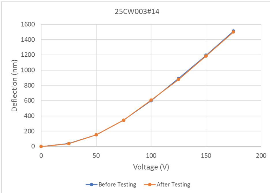
*Figure 19: Quasi-static mirror displacement data from before and after vibration exposure at GSFC testing at Princeton.*
