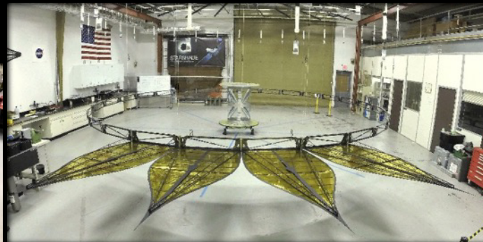
Positioning the petals to high accuracy, blocking on-axis starlight, maintaining overall shape on a highly stable structure (S-5)
