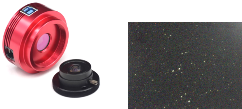
Figure 9: (Left) The ASI224MC "hockypuck" camera. The heart of the camera is the imaging sensor (shown in the center) which is supported by a round housing with a USB3 and ST4 cable port. The front of the camera is threaded to allow us to easily attach it to our imaging train. (Right) An example raw image taken with the ASI224MC. Note that your images will be monochrome before the process of debayering
