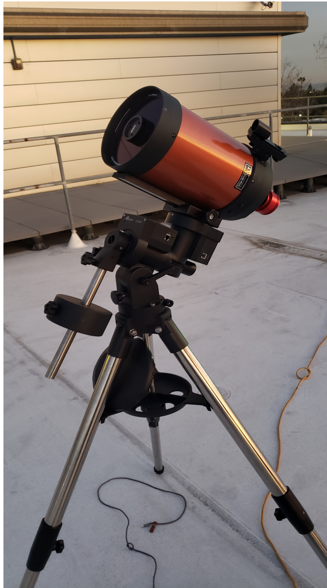
Figure 12: A fully assembled Exoplanet Watch setup ready to begin observing. Note that the tripod legs are fully extended to give room when Polar Aligning, the counterweight is properly positioned to balance the weight of the telescope tube, and the telescope itself is properly positioned on the dovetail mount.
