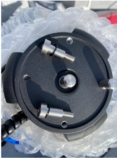
Figure 11: Tripod base and the two required bolts to mate the CEM26 Equatorial Mount. Note the locking pin located on the right-hand side. This is used to position the mount relative the the azimuth adjustment bolts and makes for a good guide when positioning the mount
