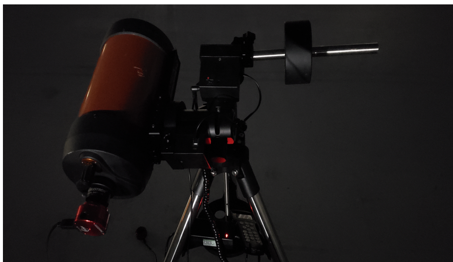
Figure 13: Equatorial Mount Balancing Position for both Right Ascension and Declination. Note that we assume the vertical Z position is already balanced, which is true for the Exoplanet Watch setup and is generally true for any telescope that is symmetric about the dovetail
