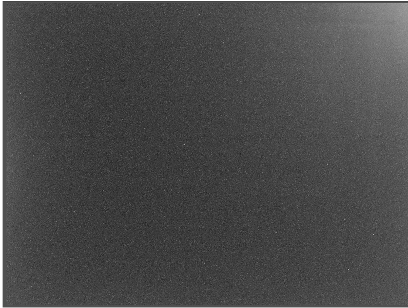
Figure 18: An example Dark frame from the ASI224MC Camera. Here the white corner "amp glow" is made obvious as well as additional "hot" and "cold" pixels
