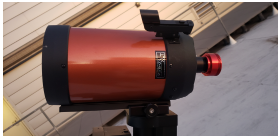
Figure 10: Existing Imaging train on an assembled observing system. Note the simple connection between visual back, nose-piece, and camera. Note that while this is a simple imaging train, other equipment combinations may have more complex considerations. If using a optical reducer or corrector, certain back-focus (distance from camera to corrector) requirements must be met. Additionally the use of any filters or guiding equipment will complicate the imaging train as well.
