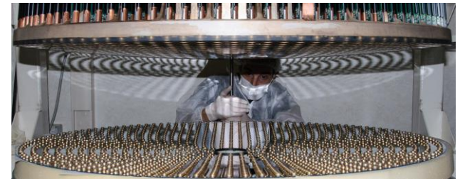
Deformable Secondary Mirror at the VLT UT-4 with 1170 actuators made by Microgate
