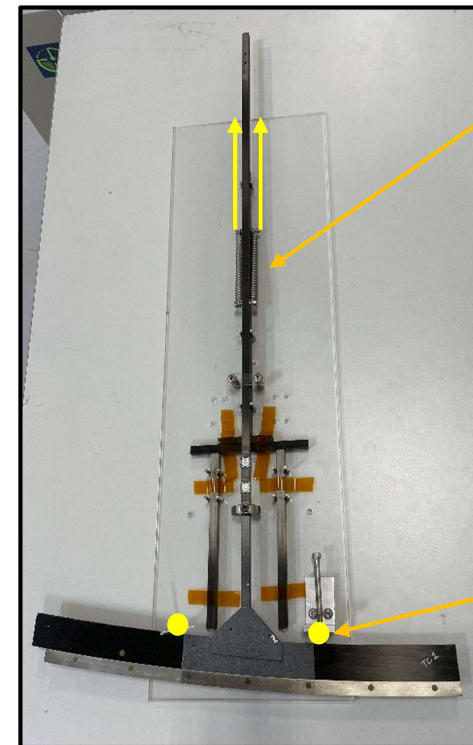
Example of a tension test load frame with joint coupon
