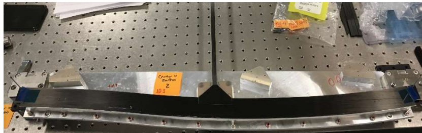
Coupon dry fit onto Protopetal fabrication fixtures
