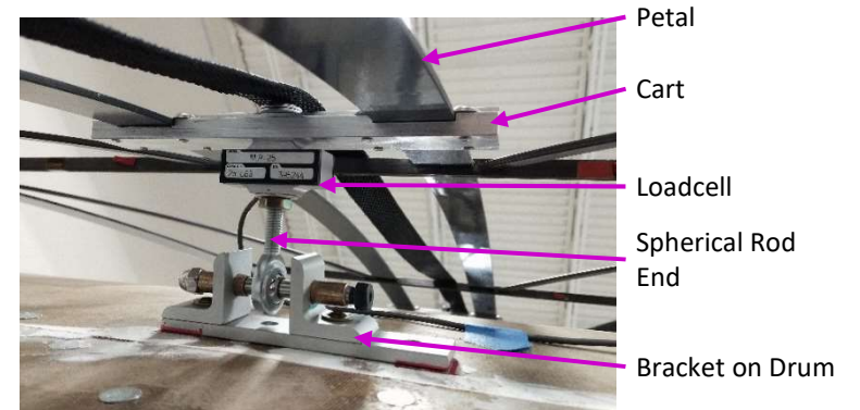
Cart on Petal Spine with Loadcell
