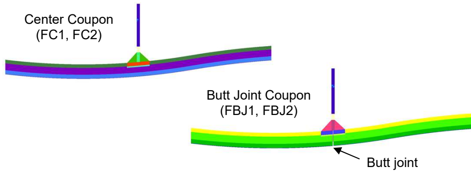
Creep Coupon Bend Test Models Extracted from Protopetal FEM
