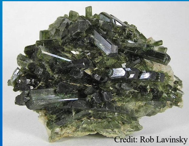
Pyroxene: \text{XY}(\text{Si}, \text{Al})_2\text{O}_6 X = Ca, Na, Fe, Mg Y = Cr, Al, Fe, Mg, Co ...
