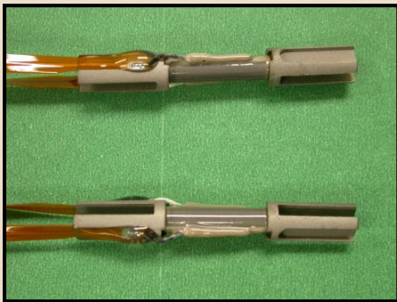
PMN actuators with titanium tabs for integration into SiC ribs
