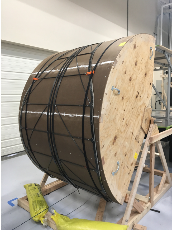
Figure 7: Prototype petal installed on the furling fixture.
