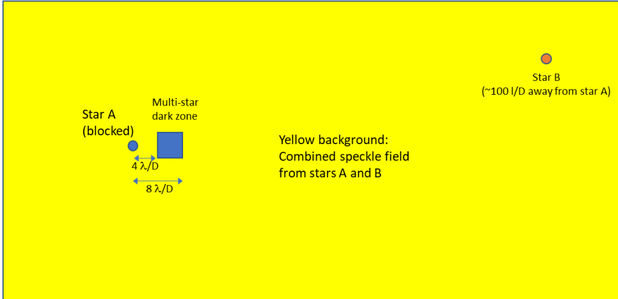
Figure 12. Schematic of the MSWC focal plane, showing the stars and the milestone dark zone. The 4-8 I/D dark zone (4x4 I/D in size) is substantially smaller than what is expected from simulations (at least 10x10 I/D in size, see Figure 6). This smaller dark zone was chosen in order to increase the confidence of achieving the milestone, but we also plan to test larger dark zones once the milestones are completed.
