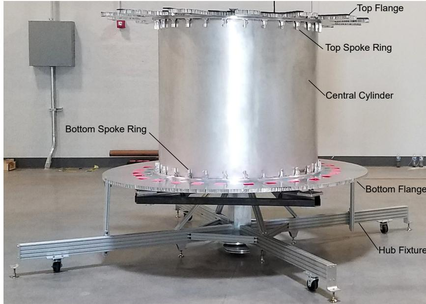
Figure 8: The structural hub and the hub fixture.
