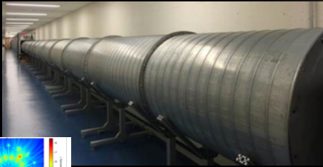
Suppressing scattered light off petal from off-axis Sunlight (S-1)
