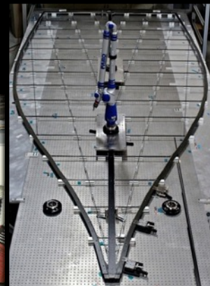
Fabricating the petals to high accuracy (S-4)
