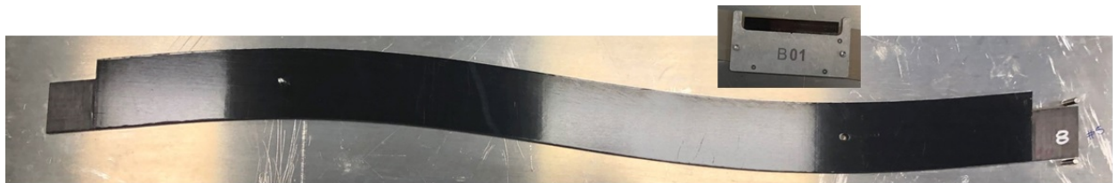
Figure 4: A 500 mm long optical edge segment. The amorphous metal edge is sandwiched between graphite composite substrates. Inset: an amorphous metal coupon mounted in its holder.
