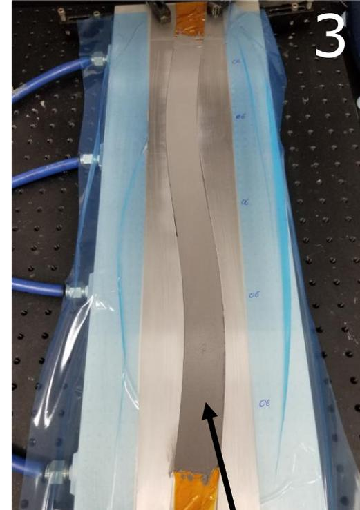
CFRP substrate post-screeding operation
