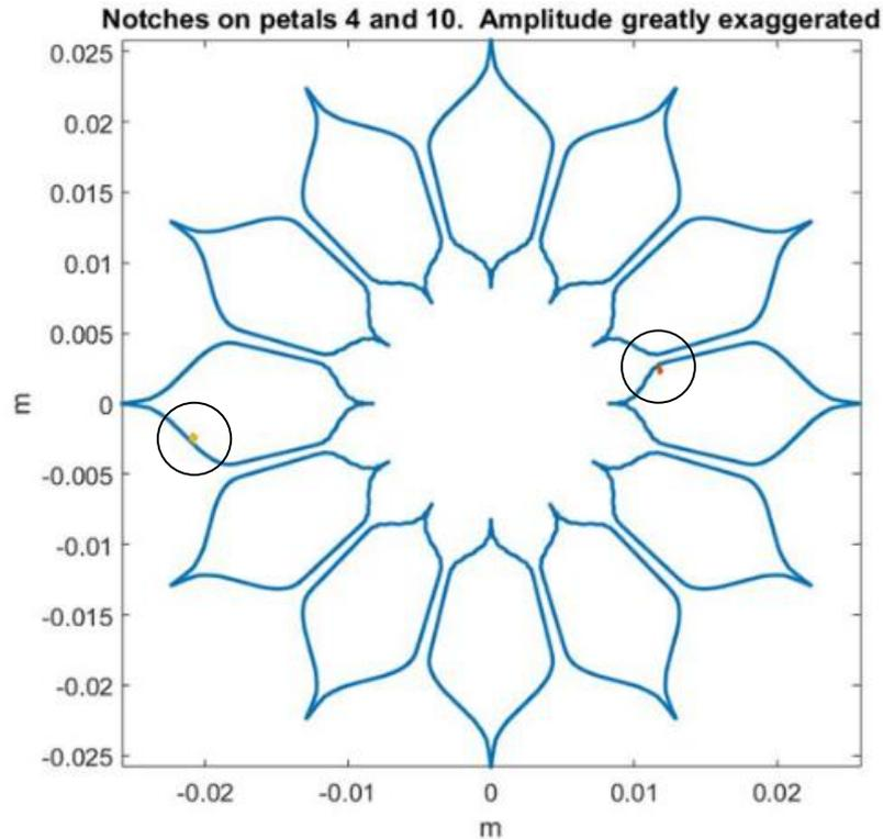
Petal edge segment displacements are modeled as 'notches' where the edge is displaced by  $\sim 2$  microns.
