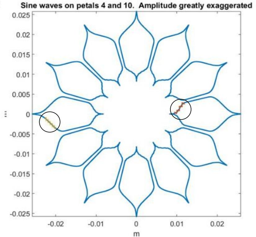
Long period sine waves with an amplitude of 1.5 microns along the petal edge. Displacement and sine amplitudes are greatly exaggerated in these plots.
