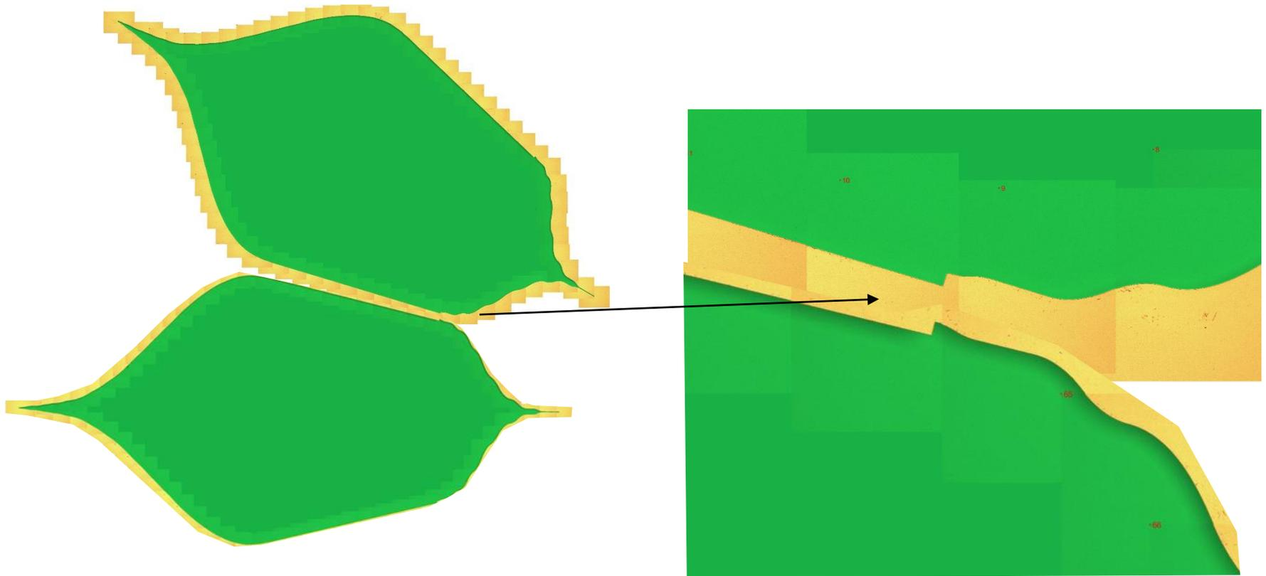
Tips are formed by rotating the outer starshade concentrically around the inner starshade to form 50  $\mu\text{m}$  wide tips.
