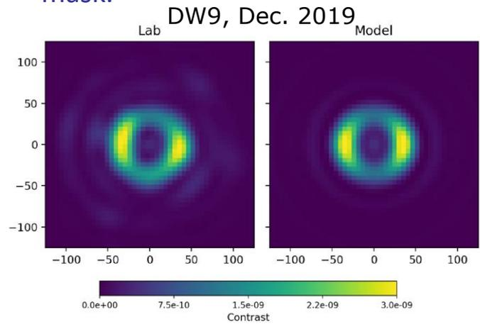
Constant Substrate Thickness of 3.23  $\mu$ m 5 Times Nominal Slope Effect Applied to Amplitude and Phase
